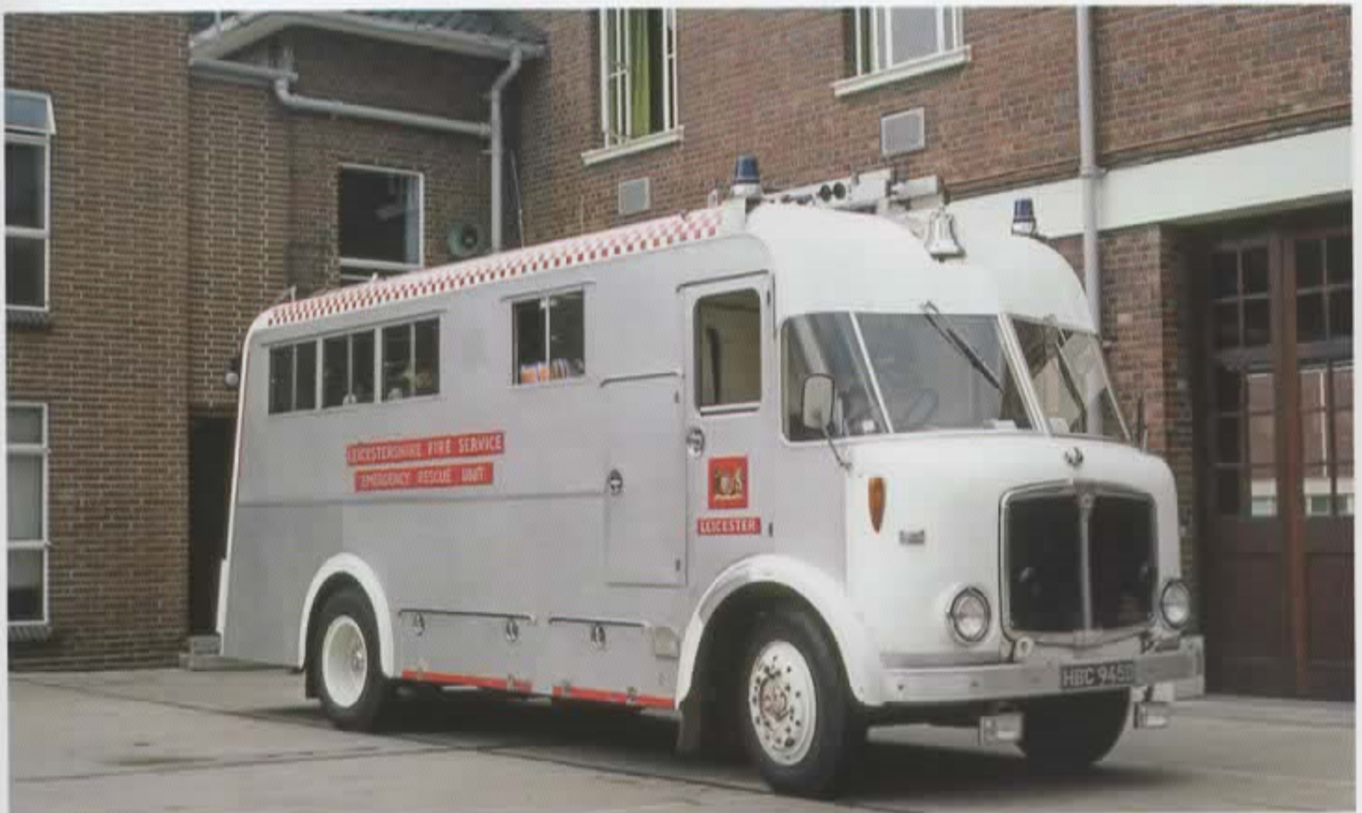
HBC 945D AEC Mercury/Merryweather ET supplied to Leicester County Borough. This type A ET passed to Leicestershire in 1974 and was apparently then known as an Emergency Rescue Unit.
