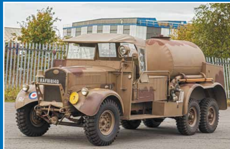
BELOW: A 'superbly preserved' Fordson 6 X 6, War Office Tender 1 (WOTI), Crash Tender, RAF108140, civilian registration RSJ 758. The later type carried 400 gallons of water and 65 gallons of foam
