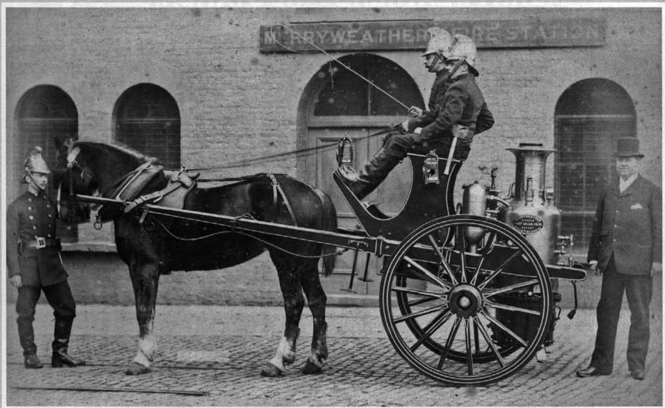
Pictured at the works and crewed by men from Merryweather's Fire Brigade, a horse drawn Valiant 'Dog Cart' steam fire engine
