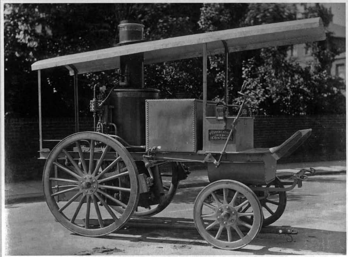
This unusual steamer for an unknown overseas customer is fitted with a sloping canopy
