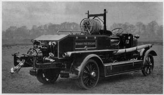
Pictured before shipping in December 1930 an Albion 30-60 turbine pump escape appliance for the Bombay Fire Brigade
