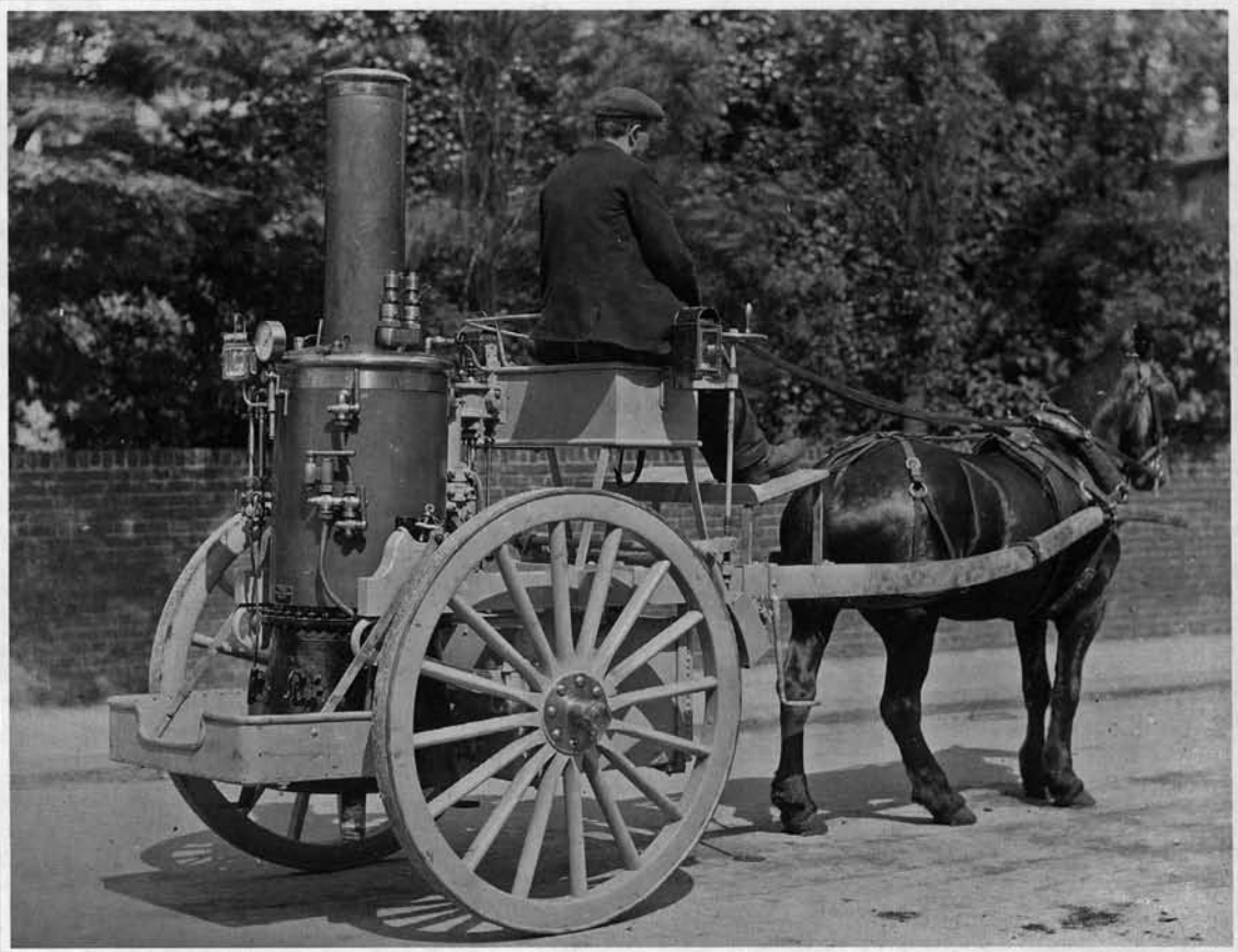
This delightful two wheeled horse drawn curricle Valiant steam fire engine was photographed on the 8th June 1911 just prior to shipping to its owners, the Italian Government
